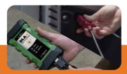
Connect your shop device to any make/model of heavy-duty vehicle using a Noregon DLA+ 3.0 Adapter.
