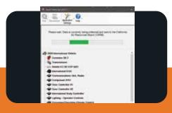
Click the Connect button to perform the scan and submit details to CARB for a pass/fail determination. Results can be viewed in the TCU Portal.
